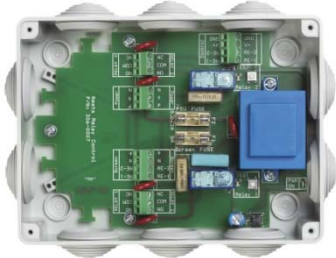
306-0007: 2 relay box with power supply
